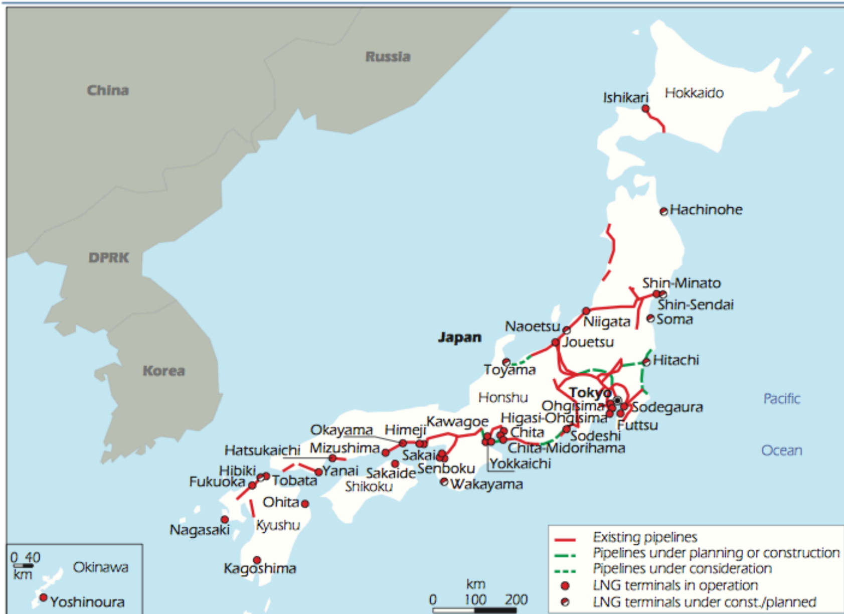
Figure 38 • LNG receiving terminals and main gas pipelines in Japan
